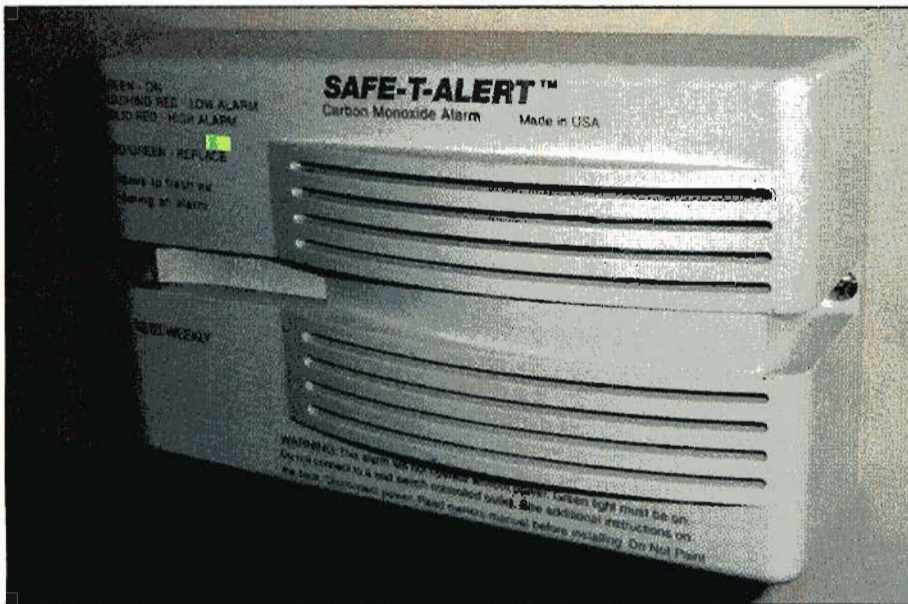
A CO detector is a "life saver." Note that the LED indicator is green. Use the test function frequently. Be sure it is wired to a circuit that is always on or, if battery-operated, install a new battery regularly.
